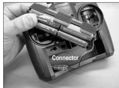
Replace the transmitter front cover and snap it closed
