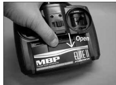
Load your Alkaline batteries into the battery holder, being very careful to put each of the batteries in the right way, as marked inside the compartments. Slide the battery holder back into position, being careful **not** to pinch the wire or loosen the connector.
