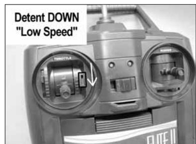
Set the boat upside down, so that the boat’s rudder and propeller are off the ground (or workbench) surface. Turn the transmitter switch to the ON position.
