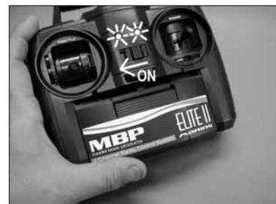
Turn on the transmitter power switch and verify that the power lights come on. Then turn the switch off. If the battery lights do not come on, open the transmitter up again and put the Alkaline batteries in the correct way before proceeding.
